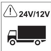
This system has been designed for the use in vehicles with an on-board supply system of 12 volts (passenger car). If you intend to install the device in a vehicle with an on-board supply system of 24 volts (lorry), please use a voltage converter. If you have queries regarding this subject, please contact our hotline.
