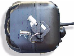
Battery backed up Siren
