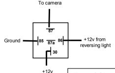
Note: Some vehicles may have computer data on the reversing light wire which may result in reduced picture quality or no picture. Check by starting the engine and engaging reverse gear. To rectify, use the reversing light voltage to control a relay (not supplied) to switch +12v to the camera.
