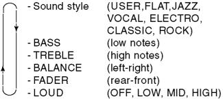
Turn the rotary knob to adjust the selected audio mode.
