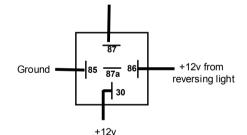
Note: Some vehicles may have computer data on the reversing light wire which may result in reduced picture quality or no picture. Check by starting the engine and engaging reverse gear. To rectify, use the reversing light voltage to control a relay (not supplied) to switch +12v to the camera.
