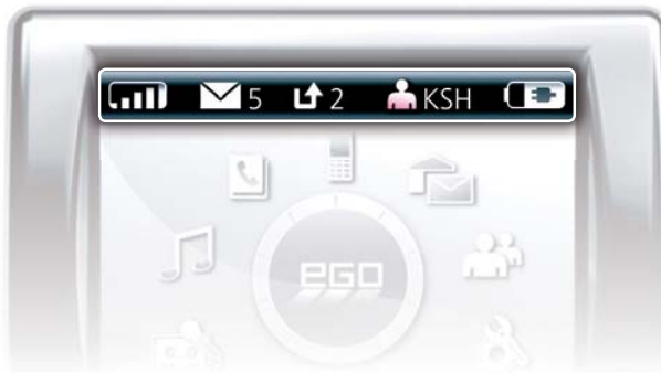
Fig. 16: Status bar The status bar is located at the top of the display and shows the symbols described in this section.
