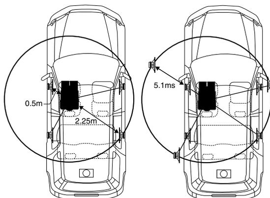
The sound is not balanced because the distance between the listening position and the various speakers is different. The difference in distance between the front left speaker and the rear right speaker is 1.75 m (68-7/8"). Here we calculate the time correction value for the front left speaker in the diagram on the above.
