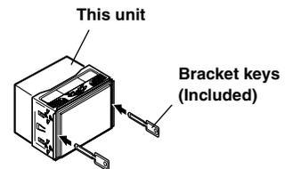
2. Pull the unit out, keeping it unlocked as you do so.
