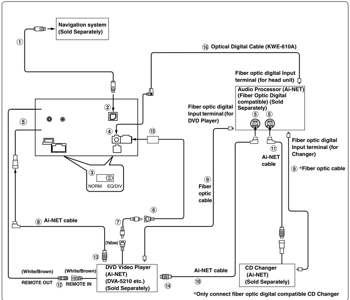
• When the fiber optic compatible product is connected, it is necessary to set the mode of this unit. Refer to “Setting the Digital Output” (page 37) and set to ON.
