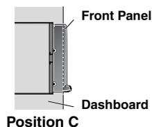
\*1 If the installed mounting sleeve is loose in the dashboard, the pressure plates may be bent slightly to remedy the problem.
