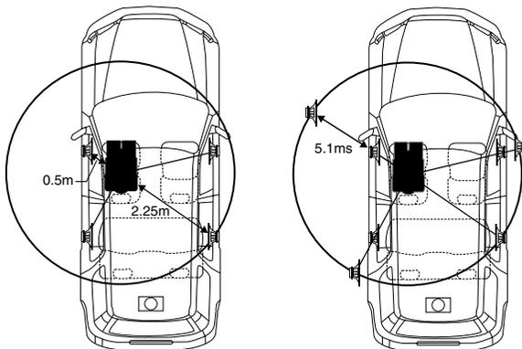
The sound is uneven because the distance between the listening position and the different speakers is different. The difference in the distance between the front left and rear right speakers is 1.75 meters (68-3/4").
