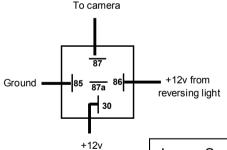
Note: Some vehicles may have computer data on the reversing light wire which may result in reduced picture quality or no picture. Check by starting the engine and engaging reverse gear. To rectify, use the reversing light voltage to control a relay (not supplied) to switch +12v to the camera.
